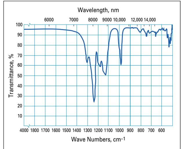
**Figure 3. Infrared Spectrum of Krytox® Grease (sodium chloride cell, capillary film). All grades of Krytox® display a spectrum similar to below.**
